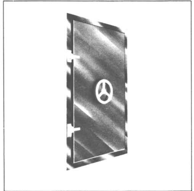
Figure I-11. Watertight Hinged Door
