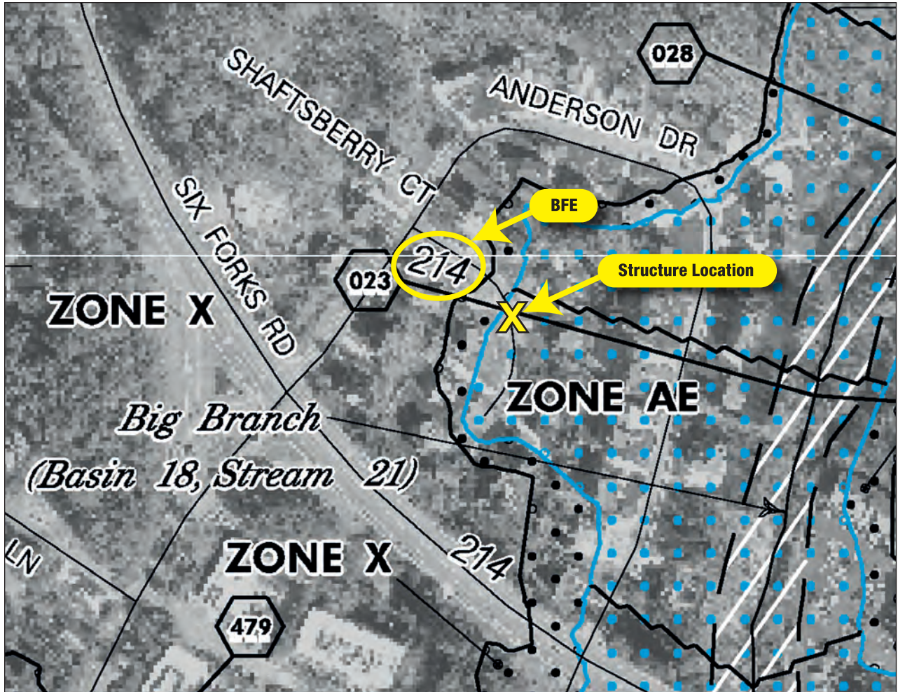
Figure 2-3. Building and stream location on a FIRM
